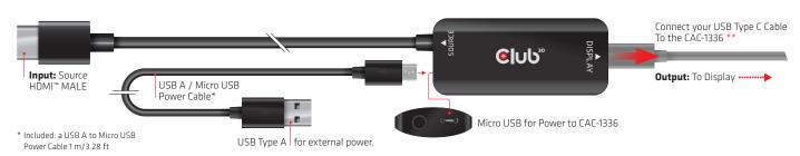
3. Connect the Power Cable with the Micro USB Connector to the CAC-1336 4. Connect the USB Type A Connector with a USB Power\*\*
